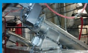
Auto-Set™ Flush Probe Installed on Screw Conveyor Discharge
