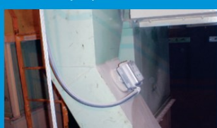
Auto-Set™ Flush Probe Installed on Belt Conveyor Discharge
