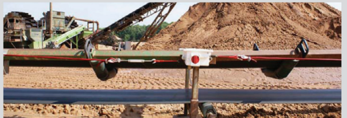
Pullswitch installed on open belt conveyor
