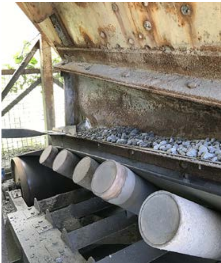
ABOVE: Before image showing the customer's spillage problem due to ineffective material containment at the transfer point.
