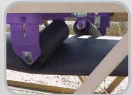
The Belt Positioner™ holds the belt in a centered position and influences the belt's path up to 2.5 M in both directions.
