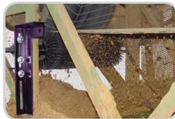
Rubber fingers create a rotary cleaning action that easily flicks carryback off the belt.
