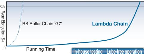
Wear elongation life is 7 times longer (14 times or more for the RS40-LMD-1 to RS60-LMD-1) than RS Roller Chains. RS120-LMD-1 and RS140-LMD-1 wear elongation life are 2.5 times longer.
