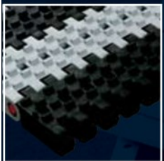
50-930 Perforated flat top surface with 3 mm staggered flight pattern. Heavy duty transport requiring drainage.
